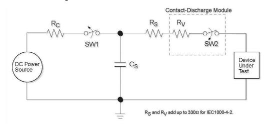
Fig. 2. ESD Test Circuit for IEC1000-4-2
