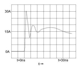
Fig. 3. ESD Test Waveform for IEC1000-4-2
