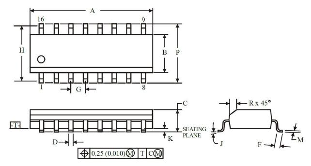
**NOTES:** 1. Dimensions A and B do not include mold flash or protrusion.
