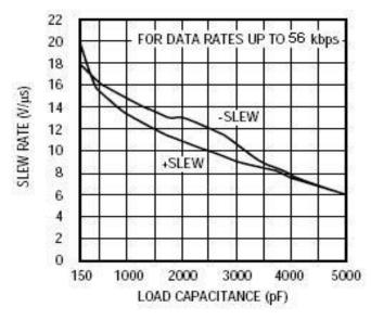
SLEW RATE vs. LOAD CAPACITANCE
