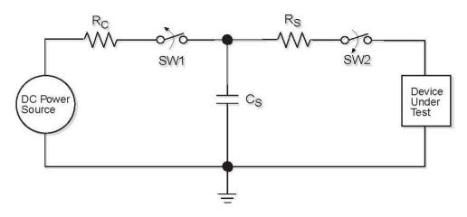
Fig. 1 ESD Test Circuit for Human Body Model
