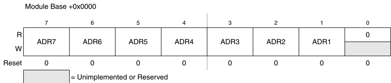
Figure 15-3. IIC Bus Address Register (IBAD)
