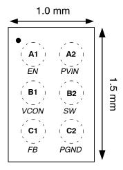
Figure 3. Pin Out (Top View)
