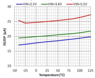
Figure 7. Sleep Mode Current vs. Temperature (EN = High, VCON = 0 V, V<sub>OUT</sub> = 0 V)
