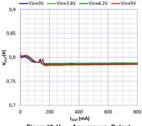
Figure 10. V<sub>OUT</sub> Accuracy vs. Output Current vs. PV<sub>IN</sub> @ 25°C, V<sub>OUT</sub> = 0.8 V
