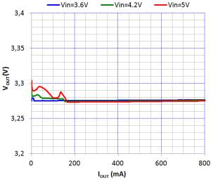
Figure 14. V<sub>OUT</sub> Accuracy vs. Output Current vs. PV<sub>IN</sub> @ 25°C, V<sub>OUT</sub> = 3.3 V
