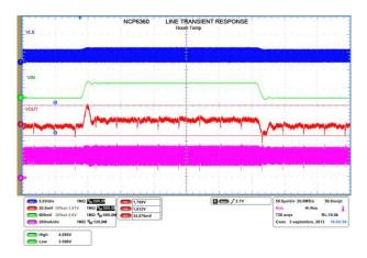
Figure 31. Line Transient Response < 20 mV Peak, PV  $_{IN}$  = 3.6 V to 4.1 V,  $R_L$  = 8  $\Omega,$   $V_{OUT}$  = 1.8 V
