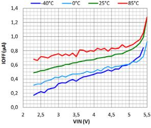
Figure 4. Shutdown Current vs Input Voltage (EN = Low, VCON = 0 V)
