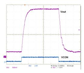
Figure 28. Transient, V<sub>OUT</sub> vs. VCON, R<sub>L</sub> = 10  $\Omega$ , V<sub>OUT</sub> = 0.4 V to 3.6 V, PV<sub>IN</sub> = 3.9 V w/ T<sub>R</sub> = 7  $\mu$ s, T<sub>F</sub> = 10  $\mu$ s
