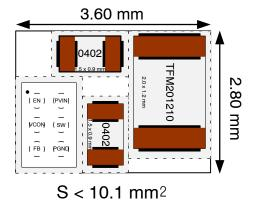
Figure 39. Layout Minimum Recommended Occupied Space Using 0402 Capacitors and 0805 (2.0 x 1.2 x 1.0 mm) Inductor
