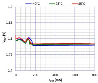
Figure 13.  $V_{OUT}$  Accuracy vs. Output Current vs. Temperature  $PV_{IN} = 3.6 \text{ V}$ ,  $V_{OUT} = 1.8 \text{ V}$
