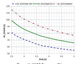
Figure 16. NMOS R<sub>DS(on)</sub> vs. PV<sub>IN</sub>
