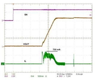
Figure 34. Power-up Transient Response PV  $_{IN}$  = 4.2 V, V  $_{OUT}$  = 3.4 V, R  $_{L}$  = 2.5 k  $\!\Omega$
