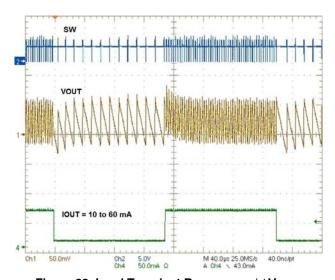
Figure 33. Load Transient Response w/  $\Delta V_{meas}$  < 50 mV Peak,  $I_{OUT}$  = 10 to 60 mA,  $V_{OUT}$  = 2.5 V
