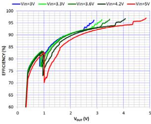
Figure 18. Efficiency vs.  $V_{OUT}$ R<sub>L</sub> = 6  $\Omega$ , Temp = 25°C
