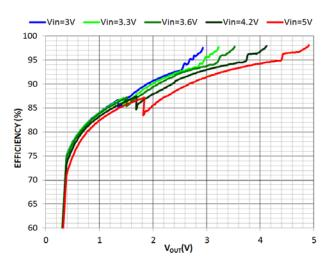
Figure 19. Efficiency vs.  $V_{OUT}$  $R_L = 10~\Omega, Temp = 25^{\circ}C$
