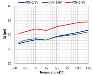
Figure 9. Quiescent Current vs Temperature  $(T_A)$ (EN = High, VCON = 0.8 V, V<sub>OUT</sub> = 2 V, no load)
