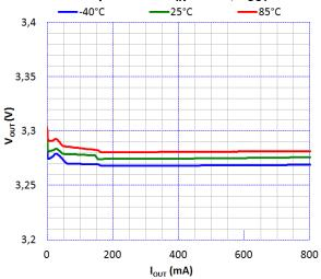
Figure 15. V<sub>OUT</sub> Accuracy vs. Output Current vs. Temperature PV<sub>IN</sub> = 4.2 V, V<sub>OUT</sub> = 3.3 V
