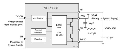
Figure 1. NCP6360 Block Diagram
