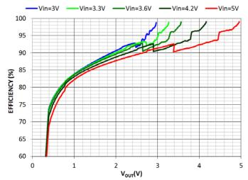
Figure 20. Efficiency vs.  $V_{OUT}$  $R_L = 22~\Omega, Temp = 25^{\circ}C$
