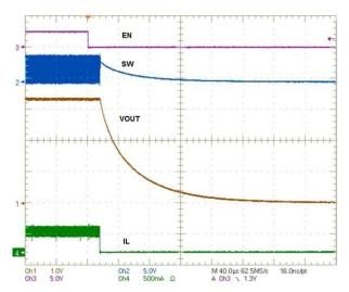
Figure 36. Power–down Transient Response PV<sub>IN</sub> = 4.2 V, V<sub>OUT</sub> = 3.4 V, R<sub>L</sub> = 10  $\Omega$
