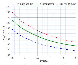
Figure 17. PMOS R<sub>DS(on)</sub> vs. PV<sub>IN</sub>
