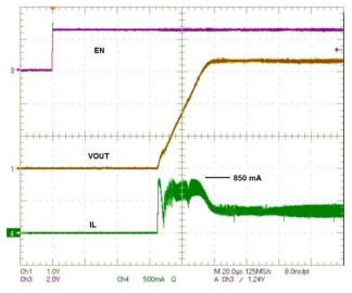
Figure 35. Power-up Transient Response PV<sub>IN</sub> = 4.2 V, V<sub>OUT</sub> = 3.4 V, R<sub>L</sub> = 10  $\Omega$
