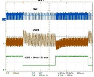
Figure 32. Load Transient Response w/  $\Delta V_{meas}$  < 50 mV Peak,  $I_{OUT}$  = 50 to 150 mA,  $V_{OUT}$  = 2.5 V
