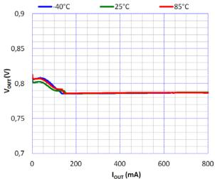
$\begin{array}{c} I_{\text{OUT}} \, (\text{mA}) \\ \text{Figure 11. V}_{\text{OUT}} \, \text{Accuracy vs. Output Current vs.} \\ \text{Temperature } \, \, \text{PV}_{\text{IN}} = 3.6 \, \text{V}, \, \text{V}_{\text{OUT}} = 0.8 \, \text{V} \end{array}$
