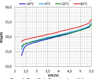
Figure 6. Sleep Mode Current vs Input Voltage (EN = High, VCON = 0 V, V<sub>OUT</sub> = 0 V)
