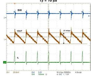
Figure 30. Output Voltage Waveforms in PFM Mode  $I_{OUT}$  = 100 mA,  $PV_{IN}$  = 3.6 V,  $V_{OUT}$  = 2.5 V,  $C_{OUT}$  = 2 x 4.7  $\mu F$
