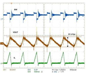
Figure 29. Output Voltage Waveforms in PFM Mode  $I_{OUT}$  = 100 mA,  $PV_{IN}$  = 3.6 V,  $V_{OUT}$  = 2.5 V,  $C_{OUT}$  = 4.7  $\mu F$
