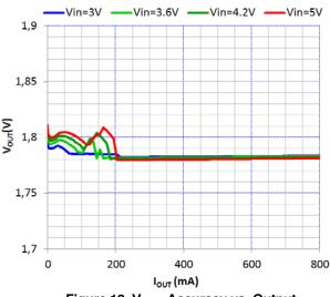
Figure 12. V<sub>OUT</sub> Accuracy vs. Output Current vs. PV<sub>IN</sub> @ 25°C, V<sub>OUT</sub> = 1.8 V
