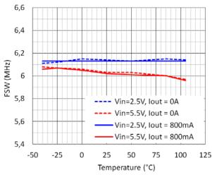
Figure 27. 6 MHz, Switching Frequency vs. Temperature (T<sub>A</sub>)
