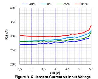
(EN = High, VCON = 0.8 V, V<sub>OUT</sub> = 2 V, no load)
