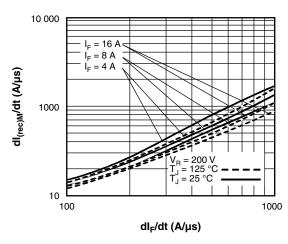
Fig. 8 - Typical dl<sub>(rec)M</sub>/dt vs. dl<sub>F</sub>/dt (Per Leg)
