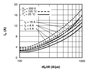
Fig. 6 - Typical Recovery Current vs. dl<sub>F</sub>/dt (Per Leg)
