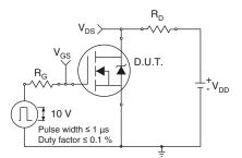
Fig. 10a - Switching Time Test Circuit
