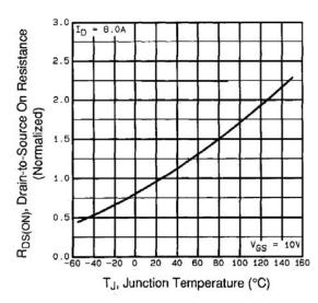
Fig. 4 - Normalized On-Resistance vs. Temperature
