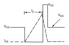
Fig. 12b - Unclamped Inductive Waveforms
