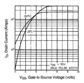
Fig. 3 - Typical Transfer Characteristics
