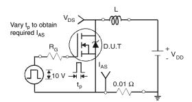
Fig. 12a - Unclamped Inductive Test Circuit
