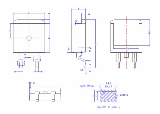
COMMON DIMENSIONS (UNITS OF MEASURE =MILLIMETER)
