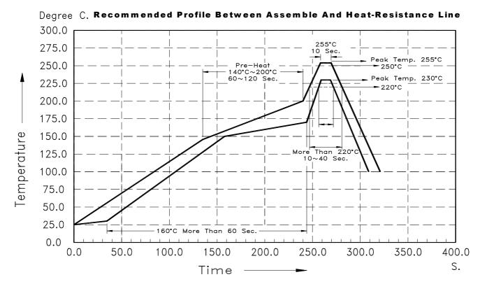
The Profile is available that must to use SnAg  $_{(\chi=3.3\sim3.8)}$  Cu  $_{(y=0.2\sim0.7)}$  solder paste
