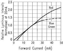
Fig.4 Relative Luminous Intensity vs. Forward Current
