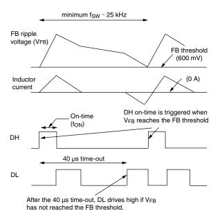
Fig. 27 - Ultrasonic Power-Save Operation
