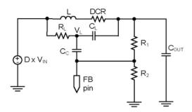
Fig. 36 - Virtual ESR Ramp Circuit
