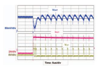
Fig. 19 - Transient Response - PSM Rising (V<sub>DD</sub> = 5 V, V<sub>IN</sub> = 12 V, V<sub>OUT</sub> = 1.5 V, I<sub>OUT</sub> = 0.5 A to 8.5 A, dI/dt = 1 A/ $\mu$ s)
