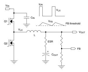
Fig. 23 - PWM Control Method, Vout Ripple
