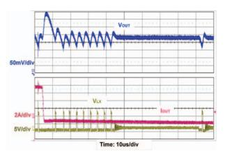
Fig. 21 - Transient Response - PSM Falling ( $V_{DD}$  = 5 V,  $V_{IN}$  = 12 V,  $V_{OUT}$  = 1.5 V,  $I_{OUT}$  = 8.5 A to 0.5 A, dI/dt = 1 A/ $\mu$ s)
