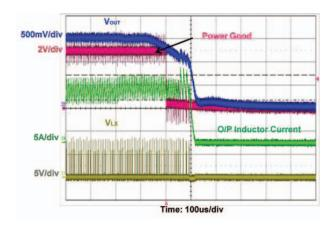
Fig. 15 - Start-Up (Pre-Bias) - EN/PSV (V<sub>DD</sub> = 5 V, V<sub>IN</sub> = 1.5 V, I<sub>OUT</sub> = 0 A)
