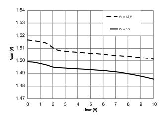
Fig. 11 - Load Regulation - PSM (V<sub>DD</sub> = 3.3 V, V<sub>OUT</sub> = 1.5 V)
