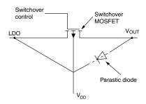
Fig. 34 - Switch-over MOSFET Parasitic Diodes
