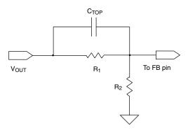
Fig. 35 - Capacitor Coupling to FB Pin
