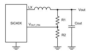
Fig. 40 - Resistor Divider Network allows 4.5 V at the V<sub>OUT</sub> Pin
