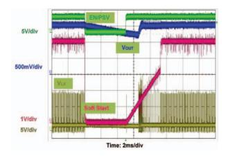
Fig. 14 - Start-Up (Pre-Bias) - EN/PSV ( $V_{DD}$  = 5 V,  $V_{IN}$  = 12 V,  $V_{OUT}$  = 1.5 V,  $I_{OUT}$  = 0 A)
