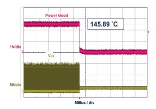
Fig. 22 - Thermal Shutdown - 146 °C ( $V_{IN}$  = 12 V,  $V_{OUT}$  = 2.5 A to 10 A, dl/dt = 1 A/ $\mu$ s)
