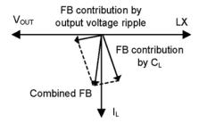
Fig. 39 - FB Voltage in Phasor Diagram
