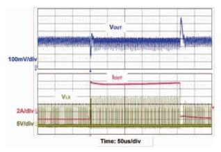
Fig. 20 - Transient Response - FCM (V<sub>DD</sub> = 5 V, V<sub>IN</sub> = 12 V, V<sub>OUT</sub> = 1.5 V, I<sub>OUT</sub> = 2.5 A to 10 A, dI/dt = 1 A/ $\mu$ s)
