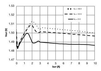
Fig. 8 - Load Regulation - PSM (V<sub>DD</sub> = 5 V, V<sub>OUT</sub> = 1.5 V)
