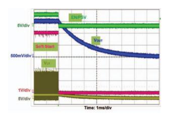
Fig. 16 - Shutdown - EN/PSV  $(V_{DD} = 5 V, V_{IN} = 1.5 V, I_{OUT} = 0 A)$
