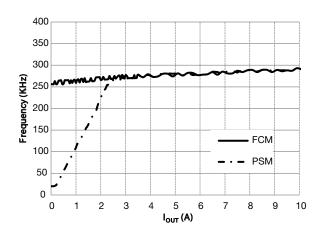
Fig. 9 - Switching Frequency - PSM vs. FCM (V<sub>DD</sub> = 5 V, V<sub>OUT</sub> = 1.5 V, V<sub>IN</sub> = 12 V)
