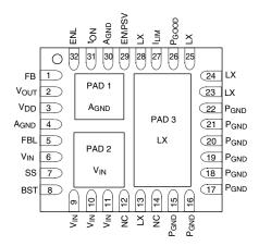
SiC402A/B Pin Configuration (Top View)
