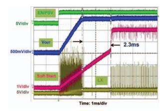
$\label{eq:fig.13-Start-Up-EN/PSV} \text{(V}_{DD} = 5 \text{ V, V}_{IN} = 12 \text{ V, V}_{OUT} = 1.5 \text{ V, I}_{OUT} = 0 \text{ A)}$
