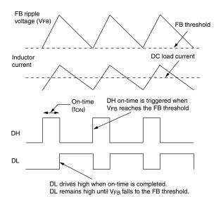
Fig. 26 - Forced Continuous Mode Operation
