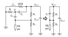
Fig. 38 - FB Voltage by Output Voltage
