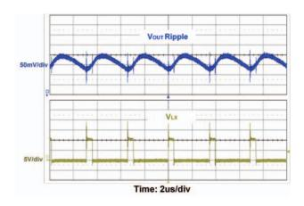
Fig. 18 - Forced Continuous Mode - SiC402ACD (V<sub>DD</sub> = 5 V, V<sub>IN</sub> = 12 V, V<sub>OUT</sub> = 1.5 V, I<sub>OUT</sub> = 10 A)
