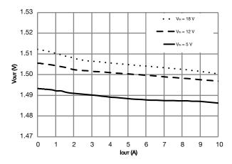
Fig. 7 - Load Regulation - FCM (V<sub>DD</sub> = 5 V, V<sub>OUT</sub> = 1.5 V)
