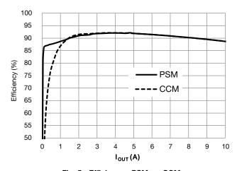
Fig. 5 - Efficiency - PSM vs. CCM ( $V_{DD}$  = 5 V,  $V_{OUT}$  = 1.5 V,  $V_{IN}$  = 12 V)
