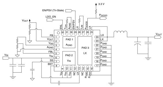
Typical Application Circuit for SiC402A/B (PowerPAK MLP55-32L)
