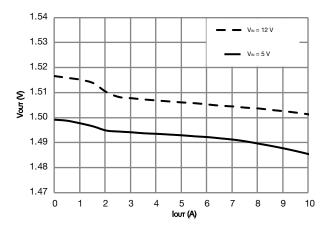
Fig. 10 - Load Regulation - FCM (V<sub>DD</sub> = 3.3 V, V<sub>OUT</sub> = 1.5 V)
