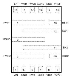
Figure 1. Top view 19-Lead QFN 3mm\*4mm
