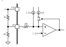
Figure 9. System UVLO by enable divider
