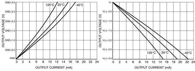
Figure 15. Negative Output Voltage Swing vs. Output Current,  $V_S = 5 \text{ V}$
