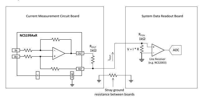
Figure 36. Remote Current Sensing
