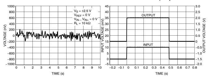
Figure 23. 0.1 Hz to 10 Hz Voltage Noise (Referred to Input)
