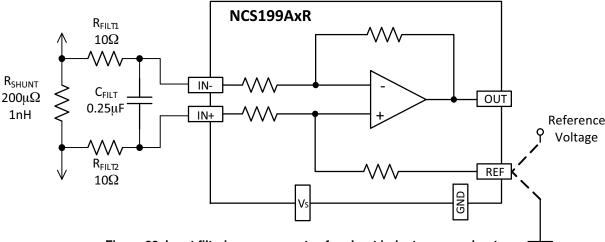
Figure 32. Input filtering compensates for shunt inductance on shunts less than 1 m $\Omega$ , as well as high frequency noise in any application
