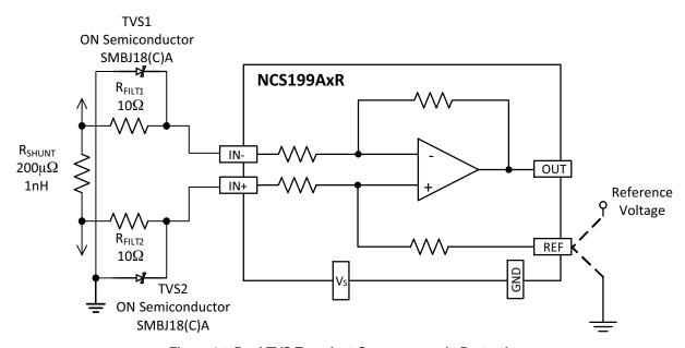
Figure 34. Dual TVS Transient Common-mode Protection
