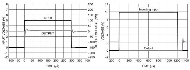
Figure 25. Common-Mode Voltage Transient Response
