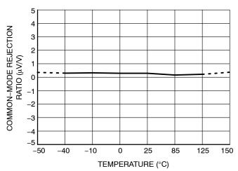
Figure 3. Common-Mode Rejection **Production Distribution**
