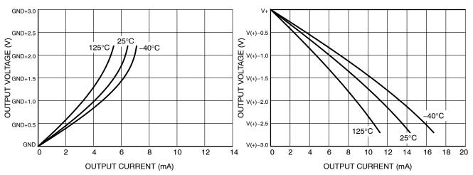
Figure 11. Negative Output Voltage Swing vs. Output Current,  $V_S = 2.2 \text{ V}$
