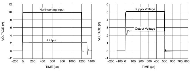
Figure 27. Noninverting Differential Input Overload
