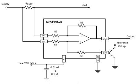
$V_{OUT} = (I_{LOAD} \times R_{SHUNT})GAIN + V_{REF}$
