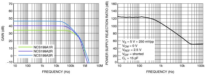
Figure 7. Gain vs. Frequency
