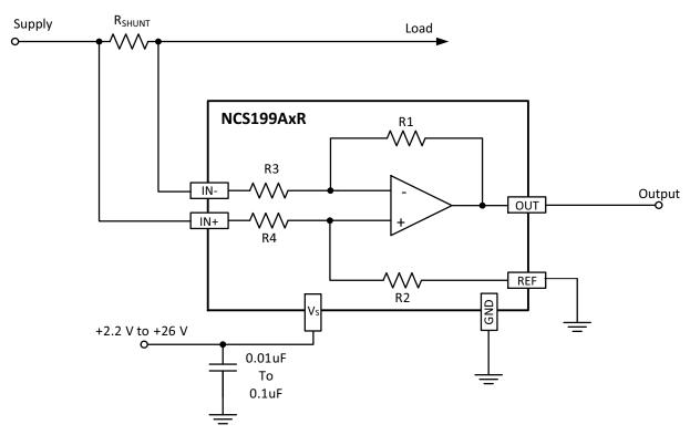
Figure 30. Basic Unidirectional Connection
