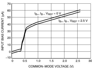
Figure 18. Input Bias Current vs. Common–Mode Voltage with  $V_S = 5 \ V$
