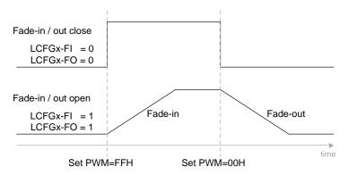
Fig8 Fade-in and Fade-out Function
