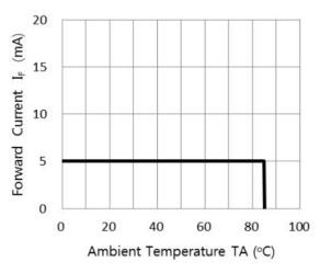
Fig. 2 FORWARD CURRENT VS. DERATING CURVE
