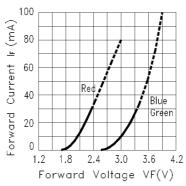
Fig.2 FORWARD CURRENT VS. FORWARD VOLTAGE
