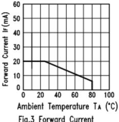
Fig.3 Forward Current Derating Curve
