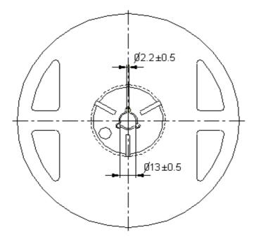
Note: 01. The tolerance unless mentioned is ±0.1mm 02. The measured unit is "mm"
