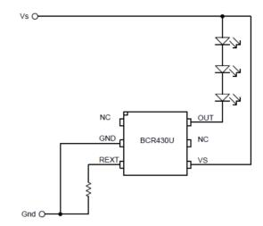
No external capacitors required for stable operation. Suitable for diming with VS or REXT pin modulation.
