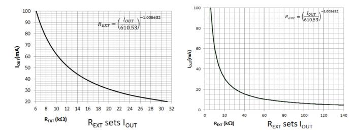
The LED current is set according to the resistor value which is connected to the REXT pin.
