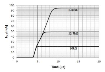
For  $R_{EXT}=6.49k\Omega$ ,  $t_R=14\mu s$  at -40°C,  $9\mu s$  at +25°C and  $7\mu s$  at +110°C. Rise time does not change significantly with LED loads (delay increases by less than  $2\mu s$ ).
