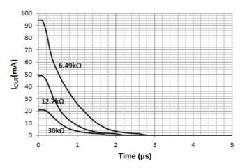
Fall time is independent of temperature. Fall time does not change significantly with LED loads.
