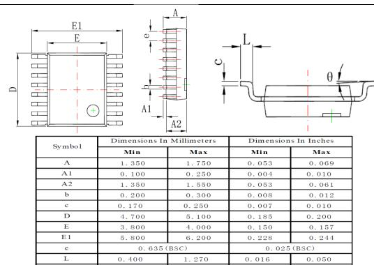
8° Figure 18.16-Lead SSOP Outline Package [SSOP16]
