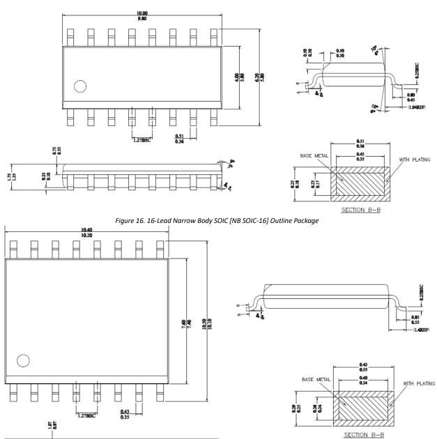
Figure 17.16-Lead Wide Body Outline Package [16-Lead SOIC\_W]
