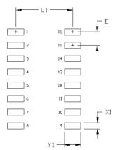
Figure 19.16-Lead Narrow Body SOIC [NB SOIC-16] Land Pattern
