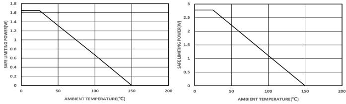
Figure 5.Thermal Derating Curve, Dependence of Safety Limiting Values with Ambient Temperature per VDE (left: π13xU3x; right: π13xU6x)
