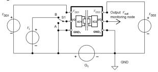
Figure 15.Common-mode transient immunity (CMTI) measurement
