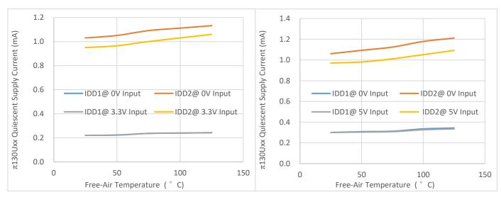
Figure 8. $\pi$ 130Uxx Quiescent Supply Current with 3.3V Supply vs. Free-Air Temperature
