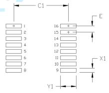
Figure 21. 16-Lead SSOP Land Pattern
