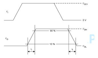
Figure 12.Transition time waveform measurement
