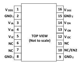
Figure  $3.\pi 130 Uxx$  Pin Configuration
