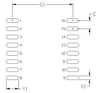
Figure 20.16-Lead Wide Body SOIC [WB SOIC-16] Land Pattern
