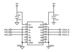
Figure 2.π130x3x Typical Application Circuit
