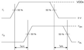
Figure 13. Propagation delay time waveform measurement
