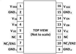
Figure 4. $\pi$ 131Uxx Pin Configuration
