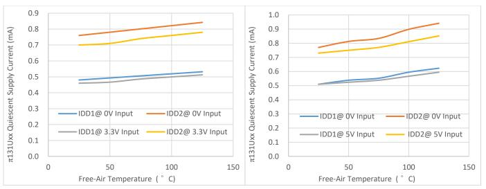
Figure  $10.\pi131Uxx$  Quiescent Supply Current with 3.3V Supply vs. Free-Air Temperature
