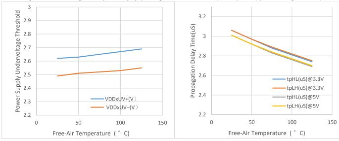
Figure 6.UVLO vs. Free-Air Temperature
