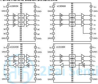
Figure  $1.\pi 130xxx/\pi 131xxx$  functional Block Diagram
