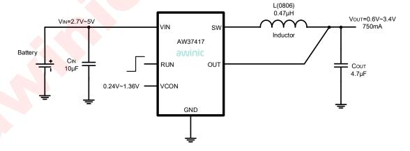
Figure 1 Typical Application Circuit of AW37417
