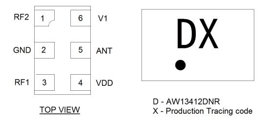
Figure 2 Pin Configuration and Top Mark
