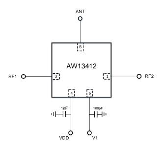
Figure 1 Typical Application Circuit of AW13412
