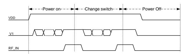
Figure 4 Power on/Change switch/Power off sequence
