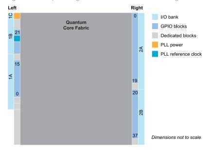
Figure 22: Floorplan Diagram for BGA49 and BGA81 Packages
