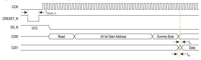
Figure 20: SPI Passive Mode (x1) Timing Sequence
