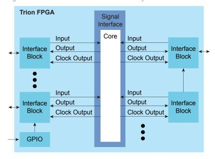
Figure 6: Interface Block and Core Connectivity
