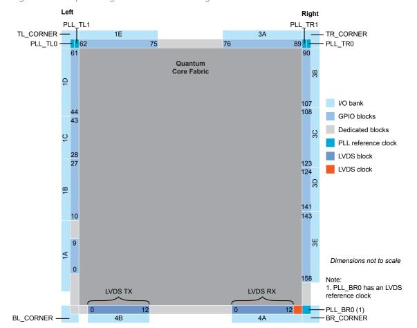
Figure 23: Floorplan Diagram for QFP144 Packages
