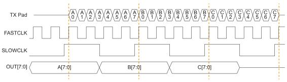
OUT is byte-aligned data passed from the core on the rising edge of SLOWCLK.
