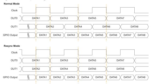
Figure 11: DDIO Output Timing Waveform
