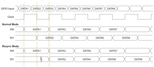
In resync mode, the IN1 data captured on the falling clock edge is delayed one half clock cycle.
