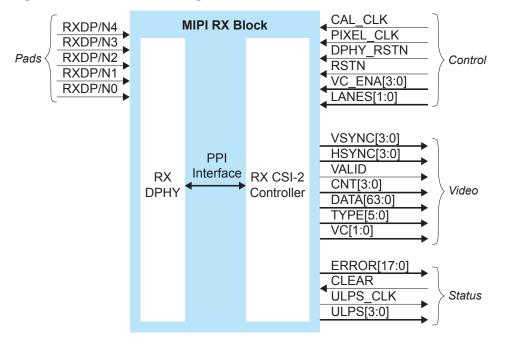
Figure 19: MIPI RX x4 Block Diagram
