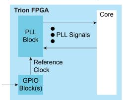
Figure 11: PLL Interface Block Diagram
