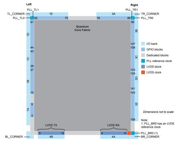
Figure 29: Floorplan Diagram for BGA256 Packages
