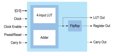
Figure 2: Logic Element Block Diagram
