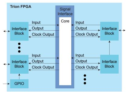
GPIO blocks are a special case because they can operate in several modes. For example, in alternate mode the GPIO signal can bypass the signal interface and directly feed another interface block. So a GPIO configured as an alternate input can be used as a PLL reference clock without going through the signal interface to the core.
