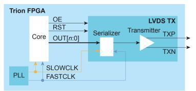
Figure 12: LVDS TX Interface Block Diagram
