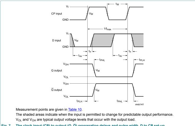
Fig. 7. The clock input (CP) to output  $(Q, \overline{Q})$  propagation delays and pulse width, D to CP set-up, CP to D hold times and the maximum frequency
