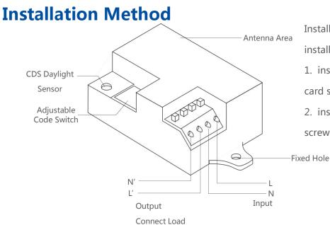
Installation Method: A variety of installation options are available: 1. install the fixed bracket with card slot and layering.
