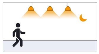
The light triggers on when the sensor detect moving object with the ambient brightness is lower than the preset threshold of photo-transistor
