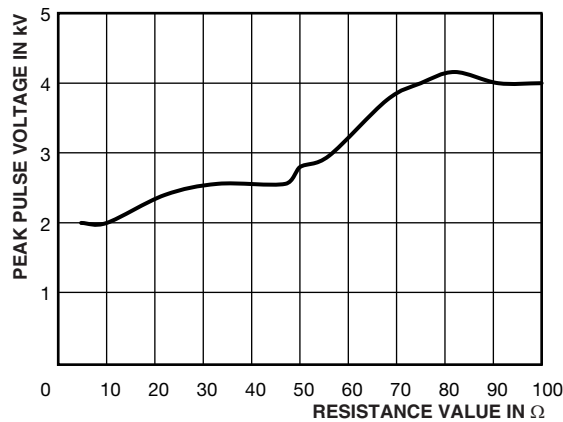
PEAK PULSE VOLTAGE LIMIT FOR AC03-CS (1.2 / 50 \mu s; 10 pulses at 30 s interval)
