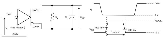
A. The input pulse is supplied by a generator having the following characteristics:  $t_r \le 6$  ns,  $t_f \le 6$  ns,  $Z_O = 50 \Omega$ .
