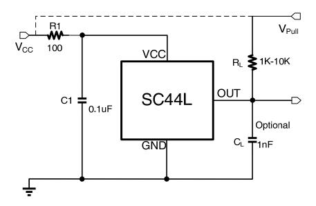
The SC44L contains an on-chip voltage regulator and can operate over a wide supply voltage range. In applications that operate the device from an unregulated power supply, transient protection must be added externally. For applications using a regulated line, EMI/RFI protection may still be required. R1 is for improved CI performance, and could be 100 or 200  $\Omega$  typically.
