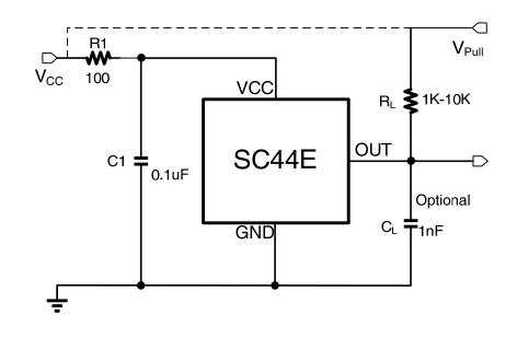
The SC44E contains an on-chip voltage regulator and can operate over a wide supply voltage range. In applications that operate the device from an unregulated power supply, transient protection must be added externally. For applications using a regulated line, EMI/RFI protection may still be required. R1 is for improved CI performance, and could be 100 or 200  $\Omega$  typically.
