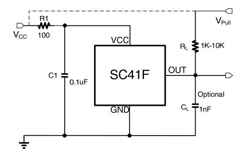
The SC41F contains an on-chip voltage regulator and can operate over a wide supply voltage range. In applications that operate the device from an unregulated power supply, transient protection must be added externally. For applications using a regulated line, EMI/RFI protection may still be required. R1 is for improved CI performance, and could be 100 or 200  $\Omega$  typically.
