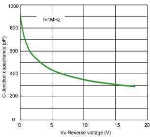
Fig 4. Capacitance vs. Reveres voltage
