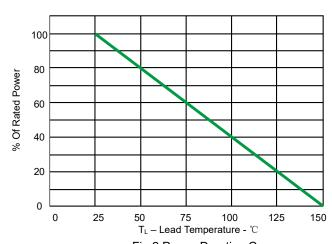
Fig 2.Power Derating Curve
