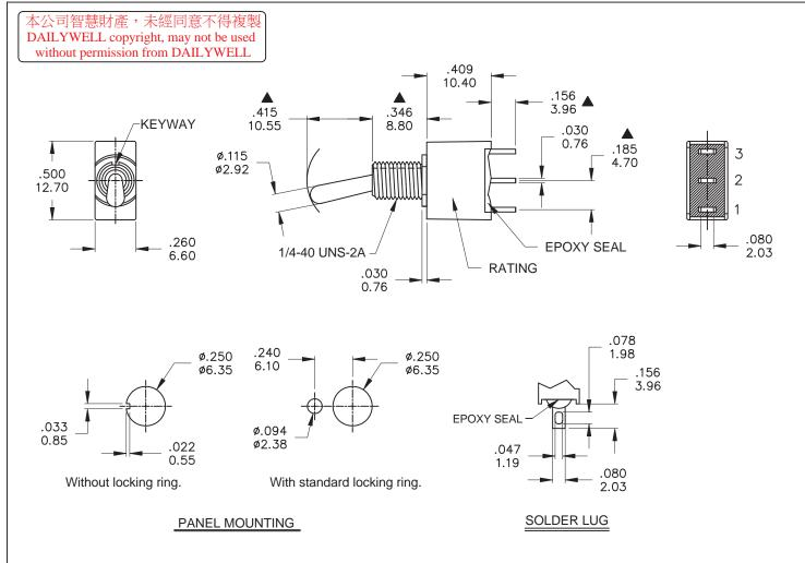
POS.3 POS.1 POS.2 Model No. ON 1AS1 ON NONE Term. 2-3 2-1 Comm. N/A 1 [ SCHEMATIC | 2 Comm.
