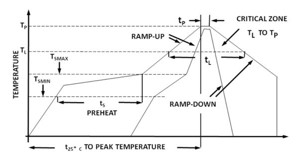
Pb-free and Sn63/Pb37 reflow profile requirements for soldering heat resistance:
