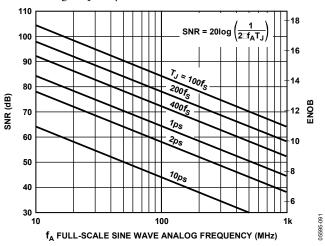
Figure 28. ENOB and SNR vs. Analog Input Frequency
