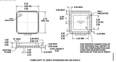
Figure 34. 32-Lead Lead Frame Chip Scale Package [LFCSP] 5 mm × 5 mm Body and 0.85 mm Package Height (CP-32-2) Dimensions shown in millimeters
