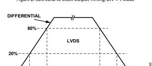
Figure 3. LVDS Timing, Differential
