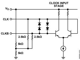
Figure 17. Clock Input Equivalent Circuit
