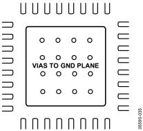
Figure 27. PCB Land for Attaching Exposed Paddle
