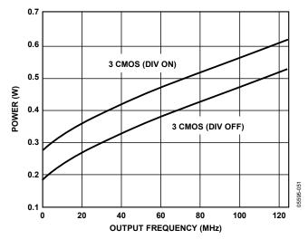
Figure 8. Power vs. Frequency—CMOS
