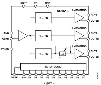
One of the outputs features a delay element with three selectable full-scale delay values (1.8 ns, 6.0 ns, and 11.6 ns), each with 16 steps of fine adjustment.
