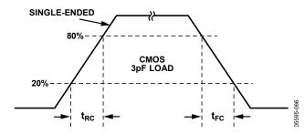
Figure 4. CMOS Timing, Single-Ended, 3 pF Load
