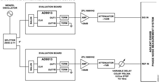
Figure 32. Additive Phase Noise Measurement Configuration
