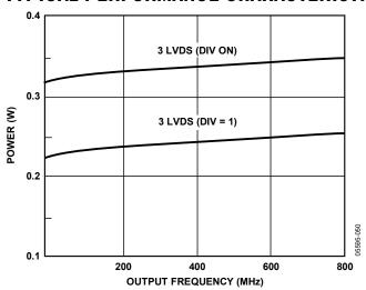
Figure 6. Power vs. Frequency—LVDS
