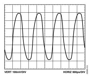
Figure 9. LVDS Differential Output at 800 MHz
