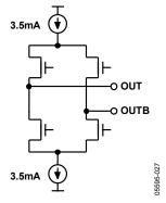
Figure 25. LVDS Output Simplified Equivalent Circuit
