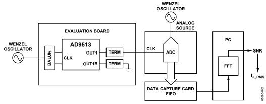
Figure 33. Jitter Determination by Measuring SNR of ADC
