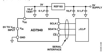
Figure 15. Typical Connection Diagram
