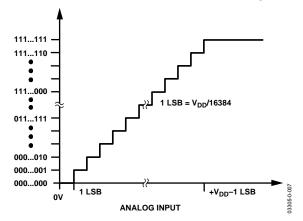
Figure 14. AD7940 Transfer Characteristic
