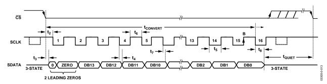
Figure 20. AD7940 Serial Interface Timing Diagram
