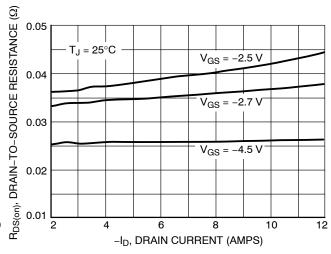
Figure 3. On-Resistance versus Gate-To-Source Voltage
