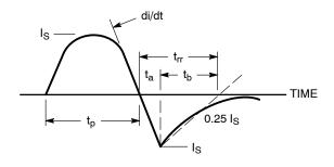
Figure 12. Diode Reverse Recovery Waveform
