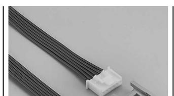
This is XM connector high box type, with 20.0mm mounting height and with 8.9mm thickness. This connector exhibits the stable electric connection to the condition such as the vibration, the prying, the micro-current and micro-voltage circuit.
