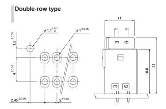
Note: 1. The above figure is the figure viewed from the connector mounting side.
