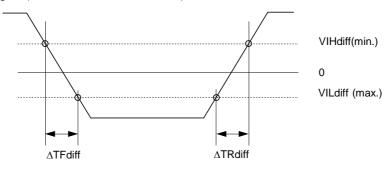
Differential Input Slew Rate Definition for DQS, /DQS and CK, /CK
