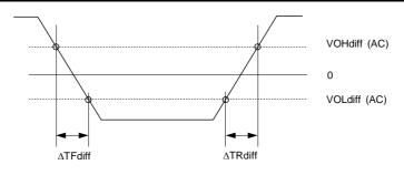
$$\text{Falling slew} = \frac{\text{VOHdiff (AC)} - \text{VOLdiff (AC)}}{\Delta \text{TFdiff}} \\ \text{Rising slew} = \frac{\text{VOHdiff (AC)} - \text{VOLdiff (AC)}}{\Delta \text{TRdiff}}$$
