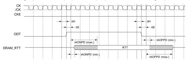
Asynchronous ODT Timings on DDR3 SDRAM with Fast ODT Transition: AL is Ignored
