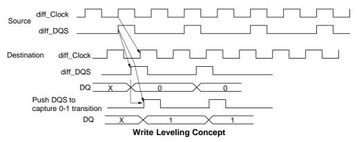
DQS, /DQS driven by the controller during leveling mode must be terminated by the DRAM, based on the ranks populated. Similarly, the DQ bus driven by the DRAM must also be terminated at the controller.
