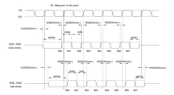
Notes: 1. Within a burst, rising strobe edge is not necessarily fixed to be always at tDQSCK (min.) or tDQSCK (max.). Instead, rising strobe edge can vary between tDQSCK (min.) and tDQSCK (max.).
