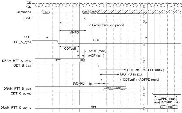
Synchronous to Asynchronous Transition During Precharge Power-Down (with DLL Frozen) Entry (AL = 0; CWL = 5; tANPD = WL - 1 = 4)
