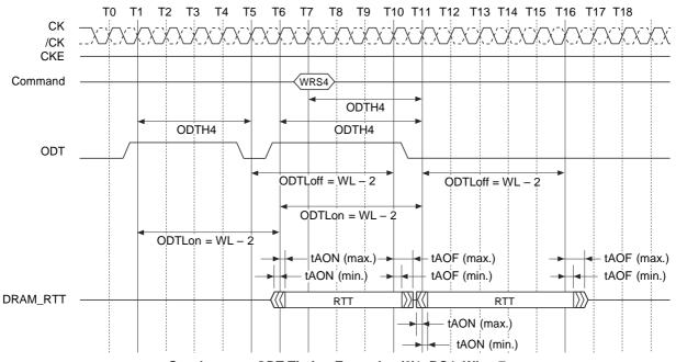
Synchronous ODT Timing Examples (2)\*: BC4, WL = 7
