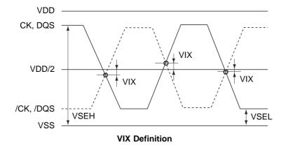
[Cross point voltage for differential input signals (CK, DQS)]
