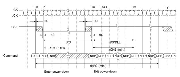
Note: \* Synchronous ODT Timing starts at the end of tXPDLL (min.)
