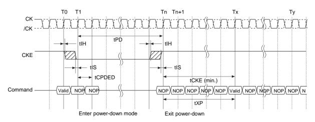
Note: Valid command at T0 is ACT, NOP, DESL or precharge with still one bank remaining open after completion of precharge command.
