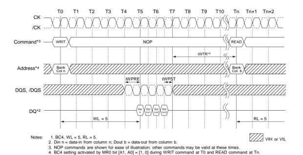
5. tWTR controls the write to read delay to the same device and starts with the first rising clock edge after
