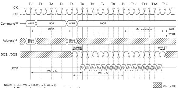
2. Din n (or b) = data-in from column n (or column b).
