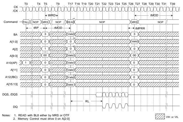
MPR Readout of Predefined Pattern, BL8 fixed Burst Order, Single Readout
