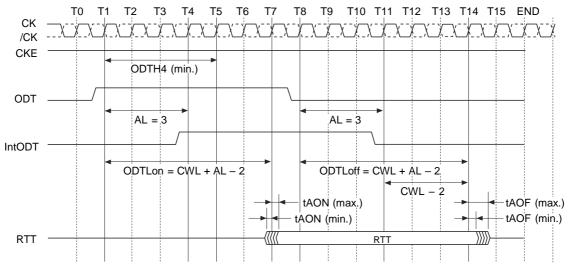
Synchronous ODT Timing Examples (1): AL=3, CWL = 5; ODTLon = AL + CWL - 2 = 6; ODTLoff = AL + CWL - 2 = 6
