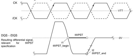
**Method for Calculating tWPST Transitions and Endpoints**
