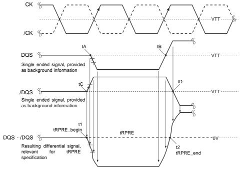
Method for Calculating tRPRE Transitions and Endpoint
