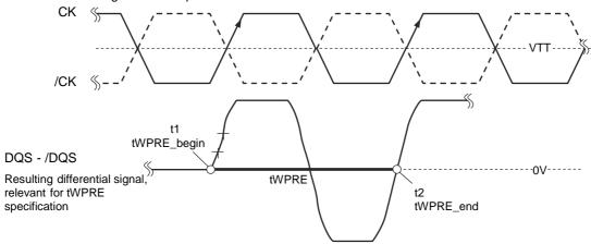
Method for Calculating tWPRE Transitions and Endpoints
