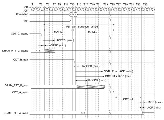
Asynchronous to Synchronous Transition during Precharge Power-Down (with DLL Frozen) Exit (CL = 6; AL = CL - 1; CWL = 5; tANPD=WL-1=9)
