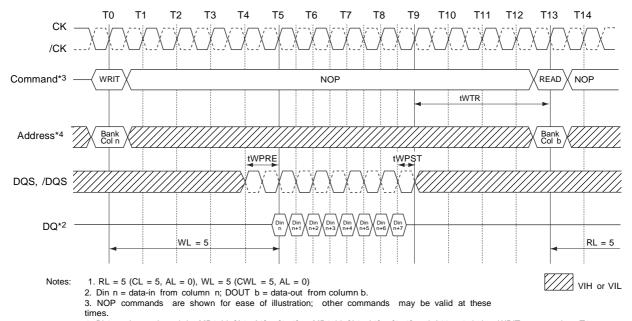
A. BL8 setting activated by MR0 bit [A1, A0] = [0, 0] or MR0 bit [A1, A0] = [0, 1] and A12 = 1 during WRIT command at T0. READ command at T13 can be either BC4 or BL8 depending on MR0 bit [A1, A0] and A12 status at T13.
