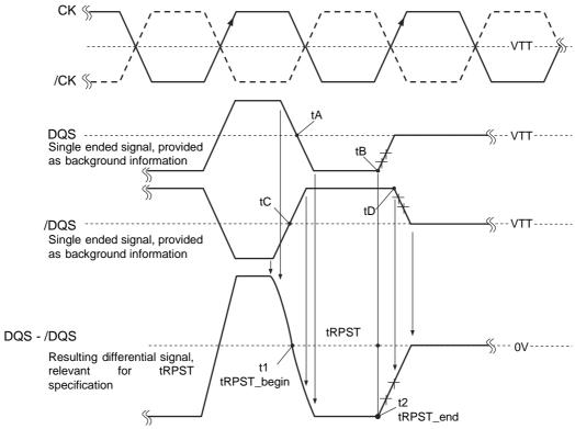
Method for Calculating tRPST Transitions and Endpoint
