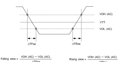
**Output Slew Rate Definition for Single-Ended Signals**
