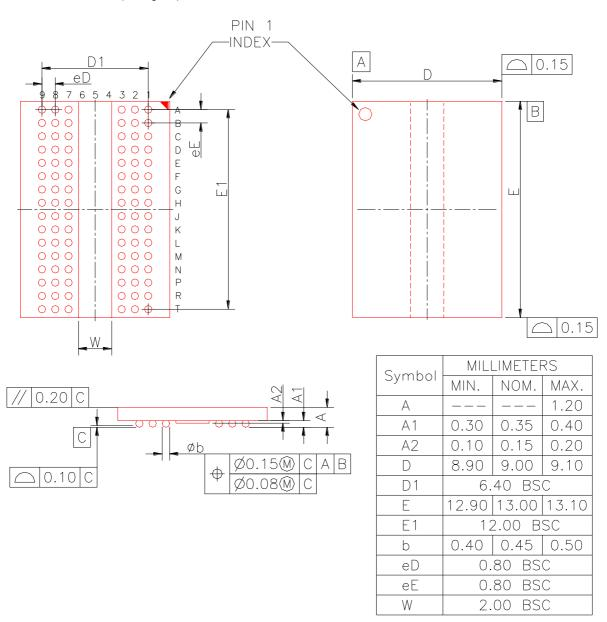
Note: The pin 1 index at buttom side is No Connection.
