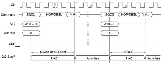
Notes: 1. CKE must be continuously registered high during the calibration procedure.
