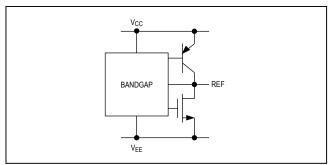
Figure 1. MAX9025/MAX9026 Voltage Reference Output Equivalent Circuit
