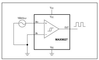
Figure 4. Zero-Crossing Detector
