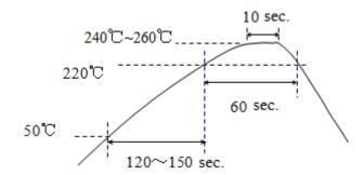
The specimen shall be passed through the reflow furnace with the condition shown in the above profile for 1 time.
