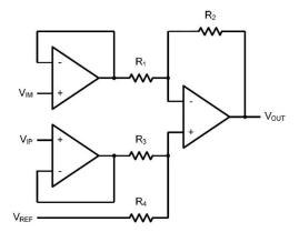
Figure 6. Instrument Amplifier
