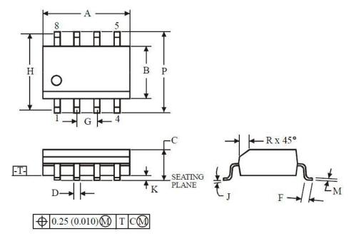
**NOTES:** 1. Dimensions A and B do not include mold flash or protrusion.
