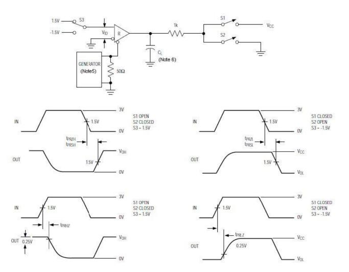
Figure 9. Receiver Enable and Disable Times
