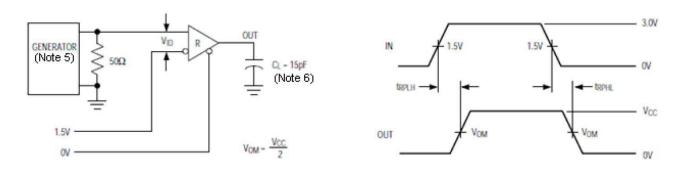
Figure 8. Receiver Propagation Delay
