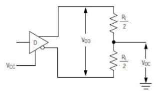
Figure 1. Driver  $V_{\text{OD}}$  and  $V_{\text{OC}}$
