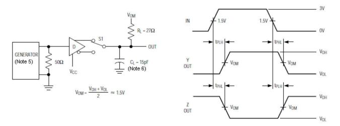
Figure 5. Driver Propagation Times
