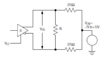
Figure 2. Driver  $V_{\text{OD}}$  with Varying Common-Mode Voltage
