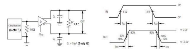
Figure 4. Driver Differential Output Delay and Transition Times
