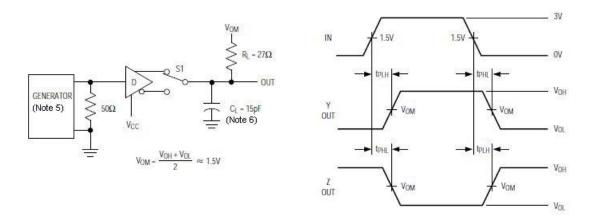
Figure 5. Driver Propagation Times
