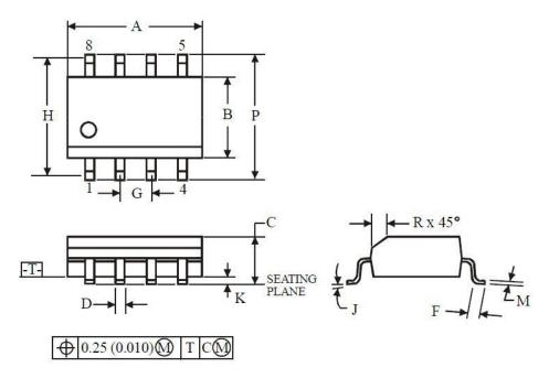
**NOTES:** 1. Dimensions A and B do not include mold flash or protrusion.
