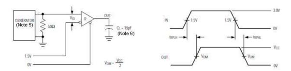
Figure 8. Receiver Propagation Delay
