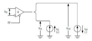
Figure 3. Receiver  $V_{\text{OH}}$  and  $V_{\text{OL}}$
