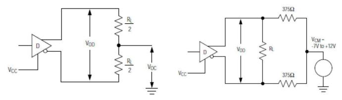
Figure 1. Driver  $V_{\text{OD}}$  and  $V_{\text{OC}}$
