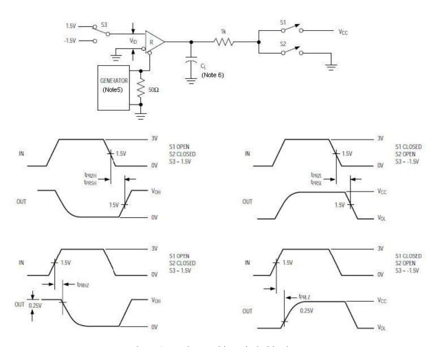
Figure 9. Receiver Enable and Disable Times
