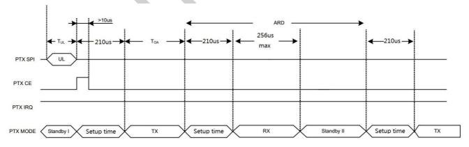
Figure 7.13Timing of Protocol engine when the first ACK packet is lost (2 Mbps)
