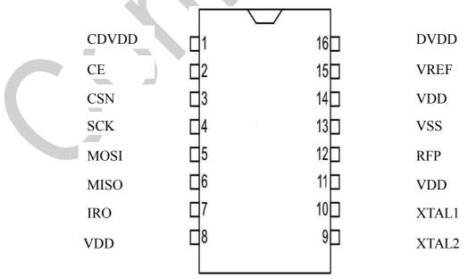
SE8R01 pin assignment (top view) for the SOP16 package
