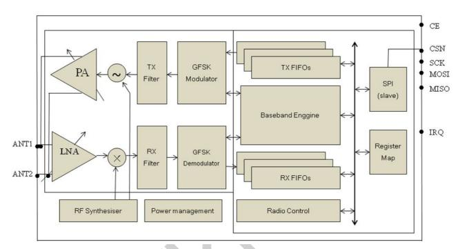
Figure1.1 SE8R01 block diagram
