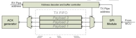
Figure 7.5TX FIFO (PRX) with pending payloads
