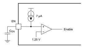
Figure 11. Capacitor Timing
