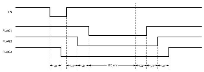
Figure 14. Incomplete Power-Down Sequence
