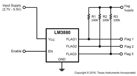
Figure 18. Sequencing Using Independent Flag Supply
