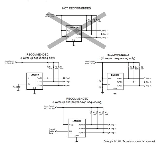
Figure 19. Recommended EN Connection
