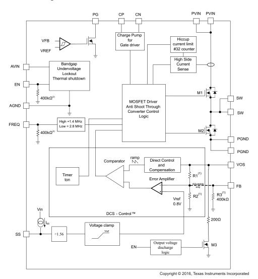
(2) The resistors are disconnected when the pins are high.
