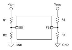
Figure 12. Output Voltage Tracking
