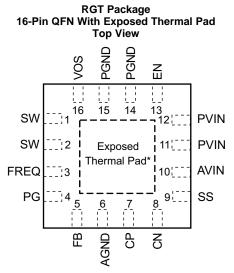
The exposed thermal pad is connected to AGND.
