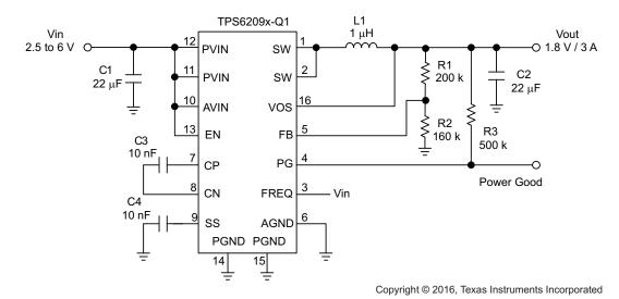
Figure 36. 1.8-V Adjustable Version Operating at 1.4 MHz
