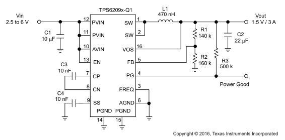
Figure 35. 1.5-V Adjustable Version Operating at 2.8 MHz
