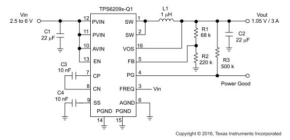
Figure 37. 1.05-V Adjustable Version Operating at 1.4 MHz
