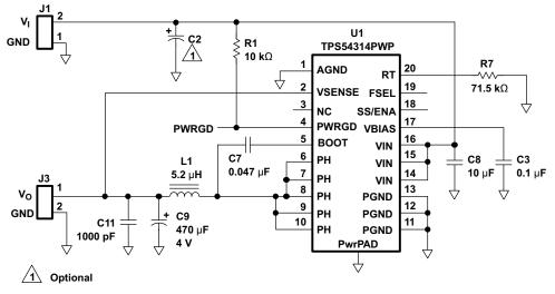
Figure 10. TPS54314 Schematic
