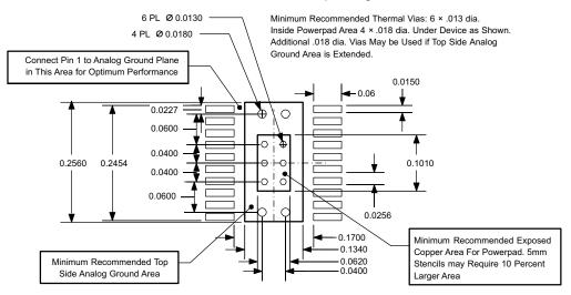
Figure 19. Recommended Land Pattern for 20-Pin PWP PowerPAD
