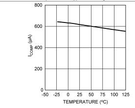
Figure 9. COMP Pin Source Current vs. Temperature
