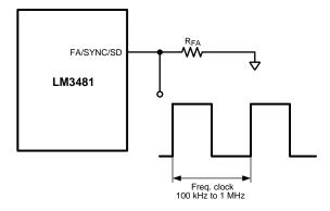
Figure 26. Frequency Synchronization
