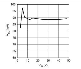
Figure 16. Compensation Ramp Amplitude vs. Input Voltage
