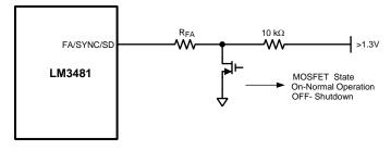
Figure 27. Shutdown Operation in Frequency Adjust Mode
