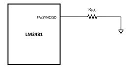
Figure 25. Frequency Adjust
