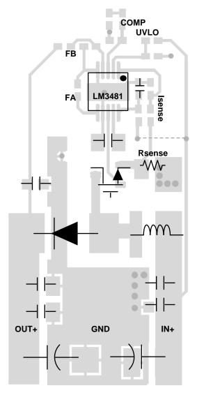
Figure 39. Typical Layout for a Boost Converter
