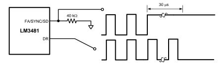
Figure 28. Shutdown Operation in Synchronization Mode
