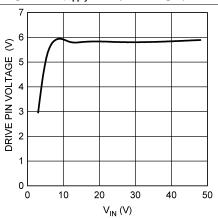
Figure 13. Drive Voltage vs. Input Voltage
