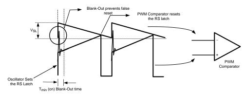
Figure 18. Basic Operation of the PWM Comparator
