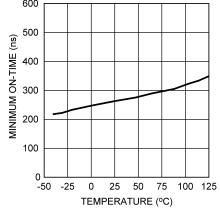
Figure 17. Minimum On-Time vs. Temperature
