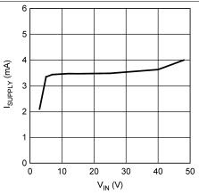
Figure 11. I<sub>Supply</sub> vs. Input Voltage (Switching)
