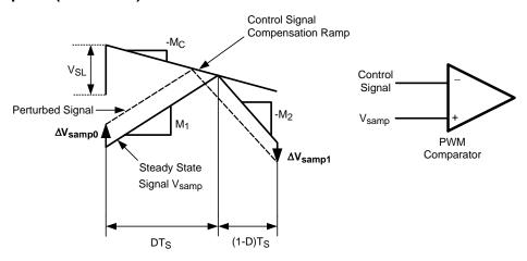
Figure 21. Compensation Ramp Avoids Subharmonic Oscillation
