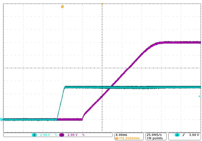
Figure 37. Start-Up Pattern for a 5-Vin, 12-Vout SEPIC Converter on LM3481 SEPIC Evaluation Module (C2: Vin, C3:Vout)
