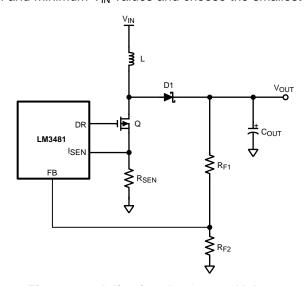
Figure 33. Adjusting the Output Voltage
