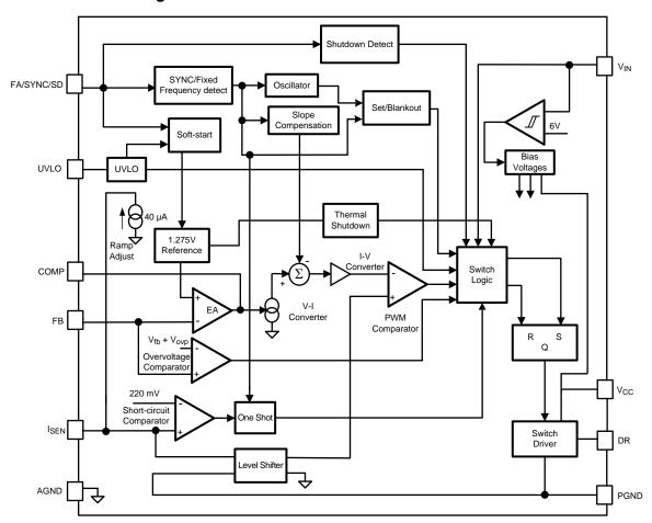
Figure 19. LM3481 Simplified Functional Block Diagram
