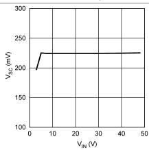
Figure 14. Short Circuit Protection vs. V<sub>IN</sub>
