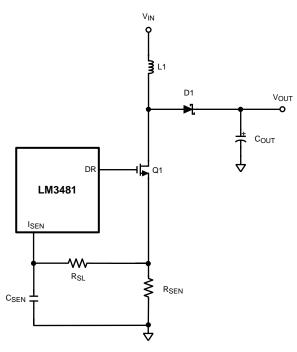
Figure 23. Increasing the Slope of the Compensation Ramp
