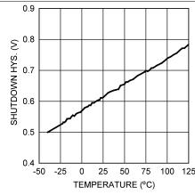
Figure 12. Shutdown Threshold Hysteresis vs. Temperature
