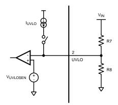
Figure 29. UVLO Pin Resistor Divider
