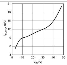
Figure 10. I<sub>Supply</sub>vs. Input Voltage (Nonswitching)
