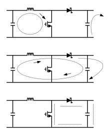
Figure 38. Current Flow in a Boost Application
