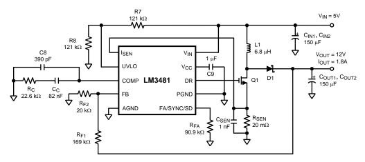
Figure 30. Typical High Efficiency Step-Up (Boost) Converter using LM3481
