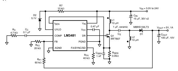
Figure 36. Typical SEPIC Converter using LM3481
