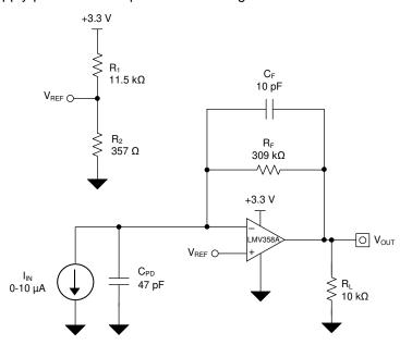
Figure 34. Single-Supply Photodiode Amplifier Circuit
