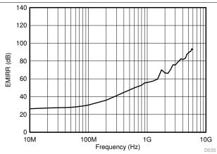
Figure 30. Electromagnetic Interference Rejection Ratio Referred to Noninverting Input (EMIRR+) vs Frequency
