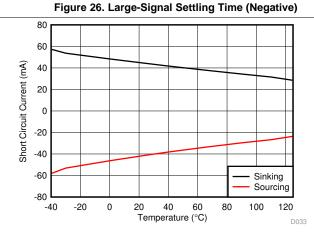
Figure 28. Short-Circuit Current vs Temperature
