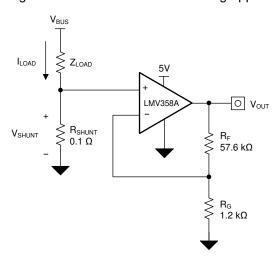
Figure 32. LMV3xxA in a Low-Side, Current-Sensing Application
