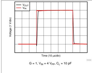
Figure 25. Large-Signal Step Response
