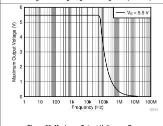
Figure 29. Maximum Output Voltage vs Frequency
