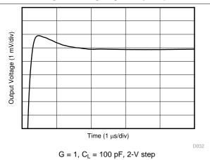
Figure 27. Large-Signal Settling Time (Positive)
