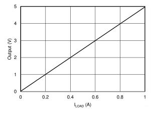
Figure 33. Low-Side, Current-Sense Transfer Function
